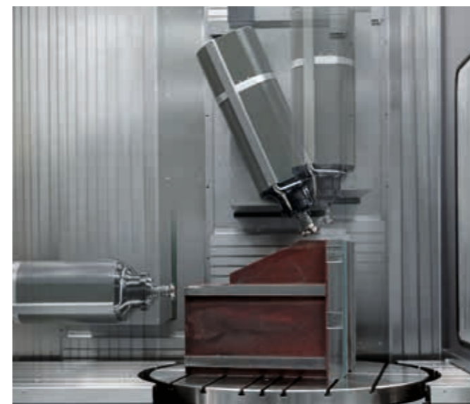
The tilting spindle head in operation: enables the machine to work in a range of ± 100°
