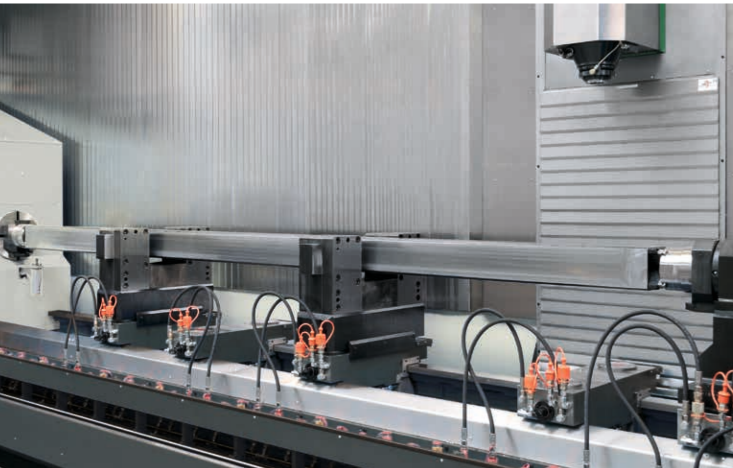
Quick set-up change from very small workpieces to very large and long workpieces by main supporting units - These can be adjusted manually in the X-direction or be NC-driven - Quickly changing clamping elements can be incorporated by the zero-point clamping systems
