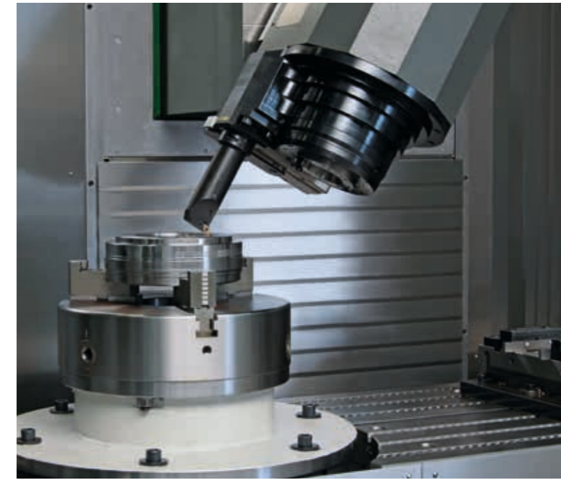
All intermediary angles can be set on the turning tool position beside the vertical and horizontal spindle position
