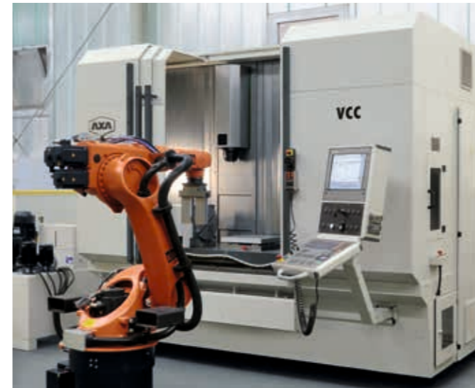
Installed industrial robot in front of the travelling column machine for direct machine loading and unloading with workpieces
