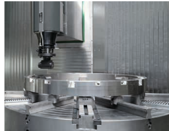
Large chucks for complete machining of rings, for example, a 6 jaw chuck with 3 centering and three adjustable jaws as well as additionally adjustable support guide-rail for the workpiece
