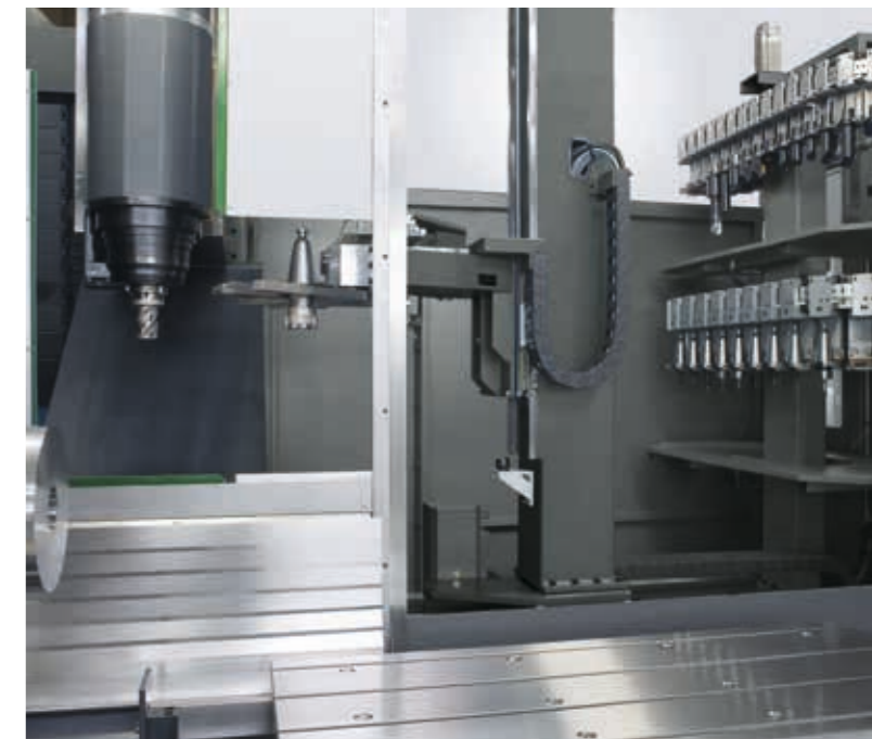
Two different tool holding fixtures can be changed by the XTS changer – for example one magazine with CAPTO C6 and a second one with SK 50
