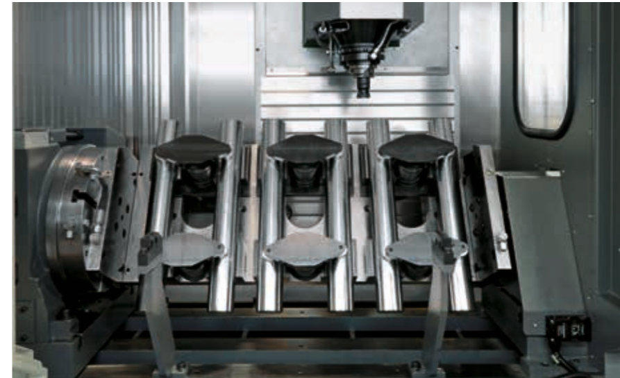
Complex hydraulic clamping unit, modularly designed by AXA, for quick conversion and secure chip flow
