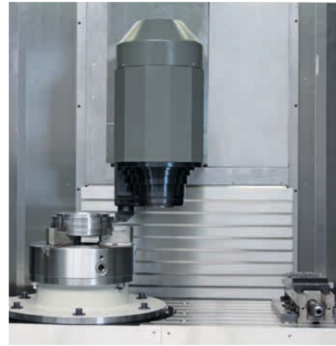
The deliberately chosen separate clamping unit for rotary tools provides optimal stability during turning machining
