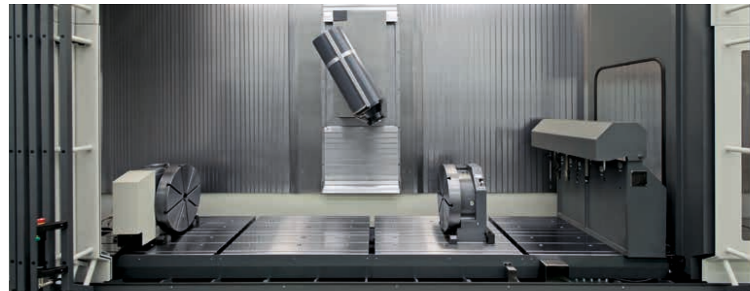
Rotary tables in gantry mode for clamping bridges as well as further, removable pick-up station left for pendulum operation or right for long bed operation
