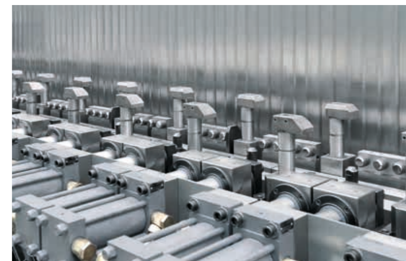
The swivel clamps are automatically moved aside during machining in the area of the milling tool and then swung back again after the machining has been completed
