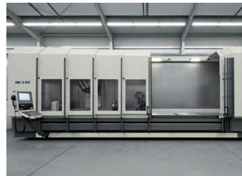
Separating the working area in two smaller ones – symmetrically, asymmetrically or with an adjustable partition wall
