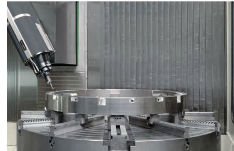
Manually adjustable jaw chuck or hydraulic jaw chuck with automatic stroke of the main jaws which are also manually adjustable
