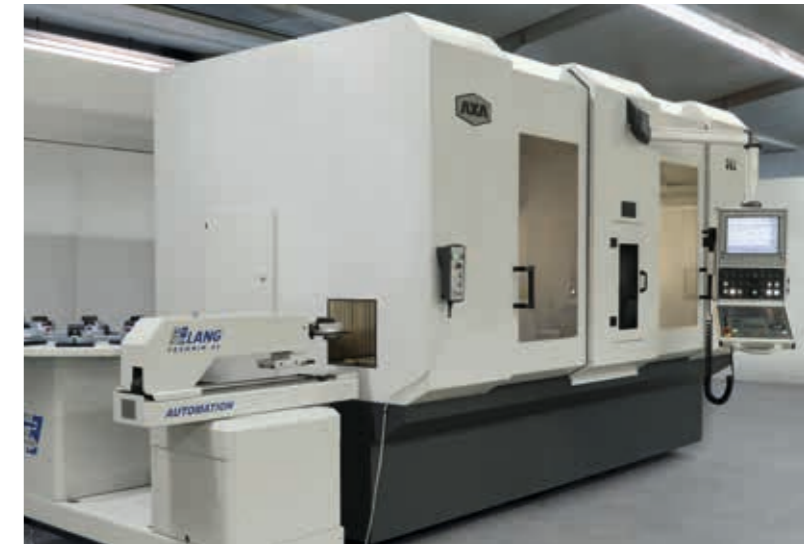
Quick and simple automisation by compact complete solution with workpiece storage, handling system and zero-point clamping
