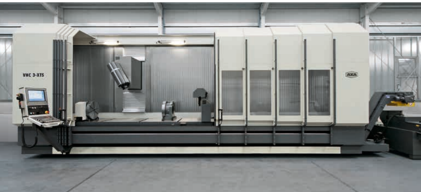
VHC travelling column machine with tilting spindle head: machining a workpiece from all sides in only one setting
