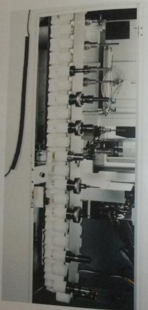
Arrangement of tools in chain-type magazine in parallel to the main spindle ensures a chip-to-chip time of 3.5 sec.
