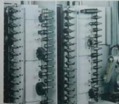
Tool tower magazine for max. 120 or 240 tools with highest tool density at minimum space requirements
