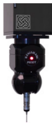
PH10T probe head fitted with TP20 probe
