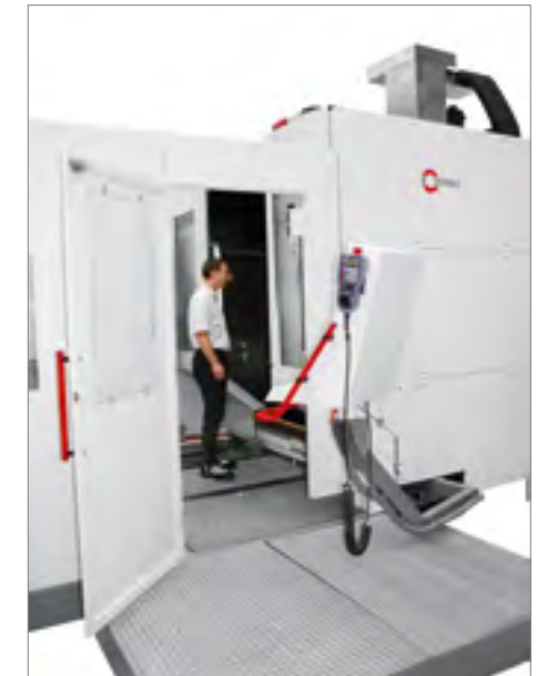
Side access to the working area of the C 50 U for manual operations or in setup mode.
