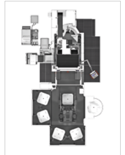
Pallet changer PW 3000 with two 2/4-pallet storage modules and setup station module, right
