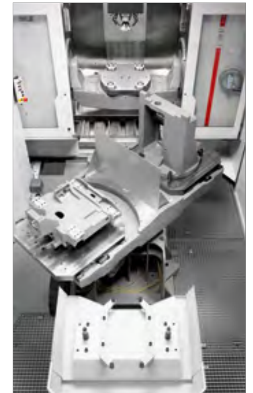
The PW 2000 can move up to 2000 kg including pallet from the setup station to the working area of the C 50 U.
