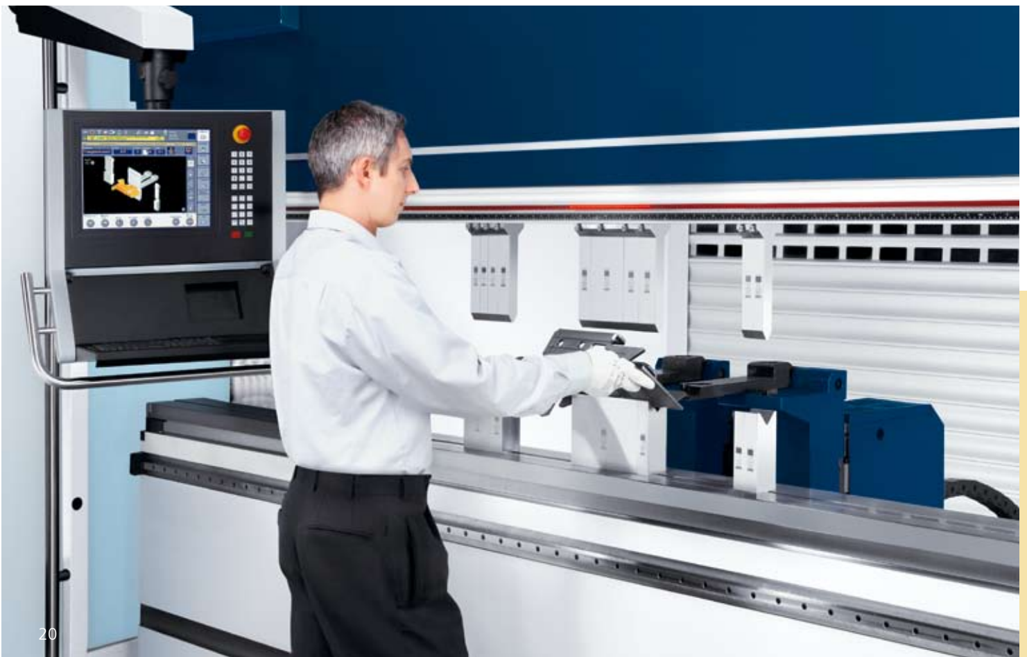
The optical positioning aid guides you from station to station.
