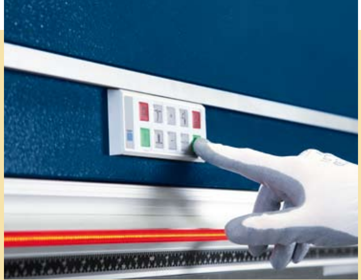
The Mobile Control unit contains the most important functions for machine control.
