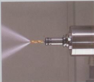
Through the spindle coolant system
