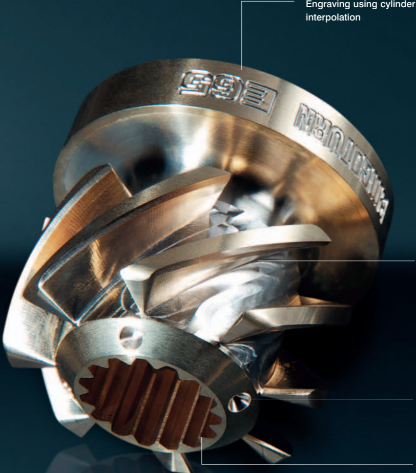
Contour milled using cylinder interpolation
