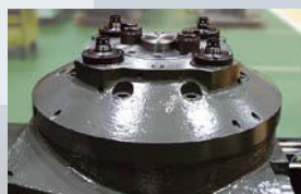
Taper-type pallet clamping mechanism
