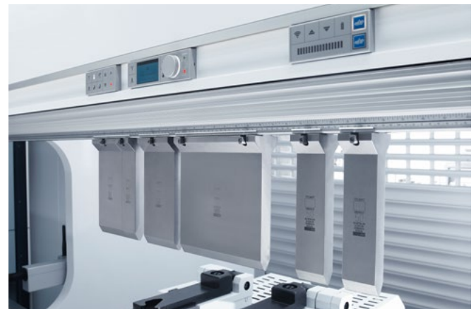
During set up the Tool Indicator shows precisely where the bending tools have to be used.
