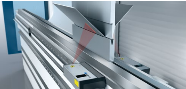
Precise angles due to laser measurement – ACB Laser.
