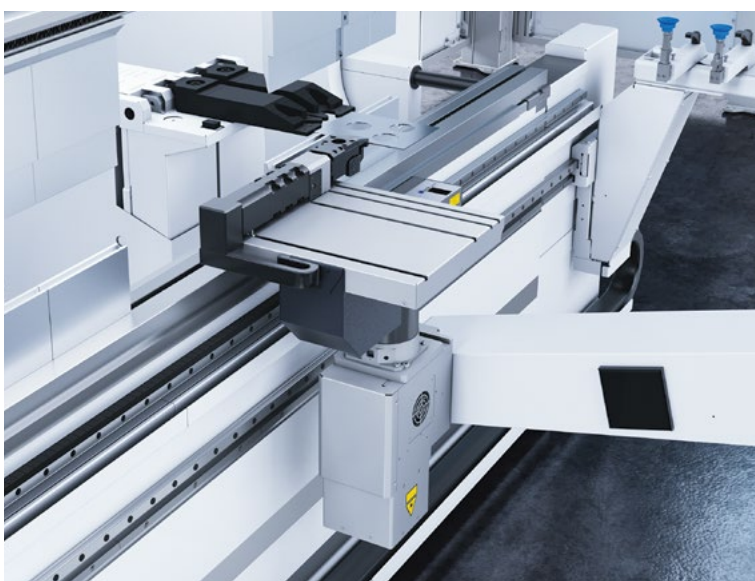
Pivoted-jaw gripper with moving and rotary axis
