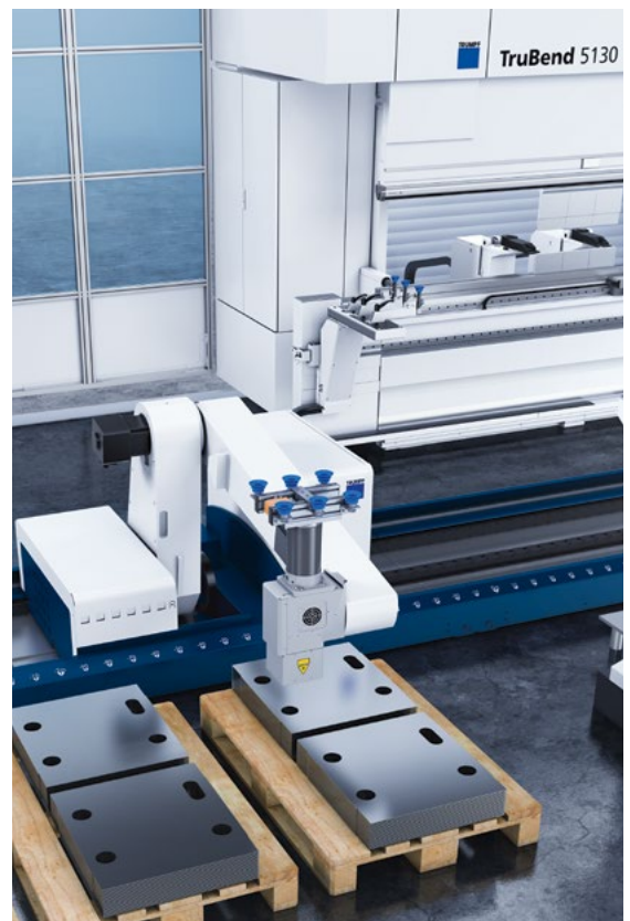
BendMaster (60) with fine-position recognition
