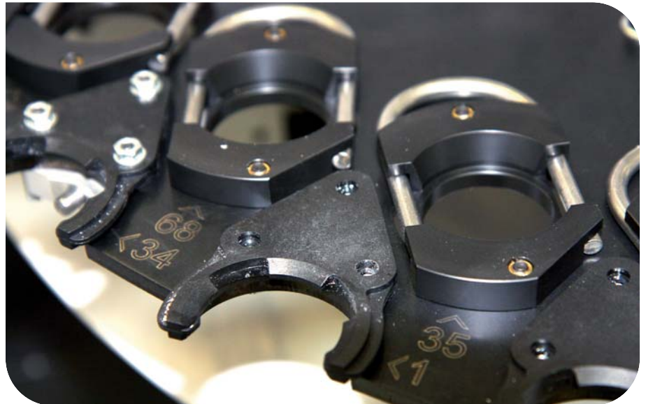
Double-row HSK-E40 magazine with a capacity of 68 tools
