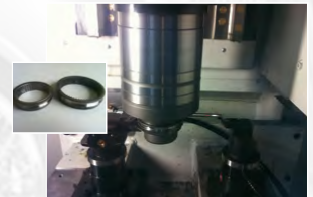
DZS 200-2 with block tools for synchronous processing of hardened sliding sleeves
