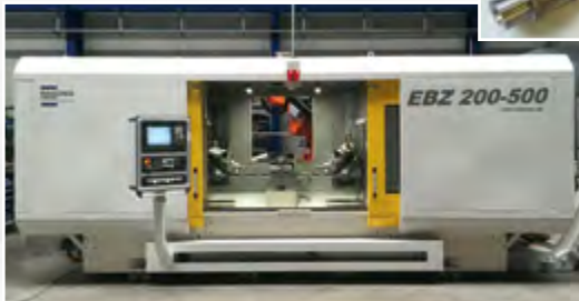
The highly productive RASOMA end-machining center EBZ 200-500, equipped with robot for loading & unloading
