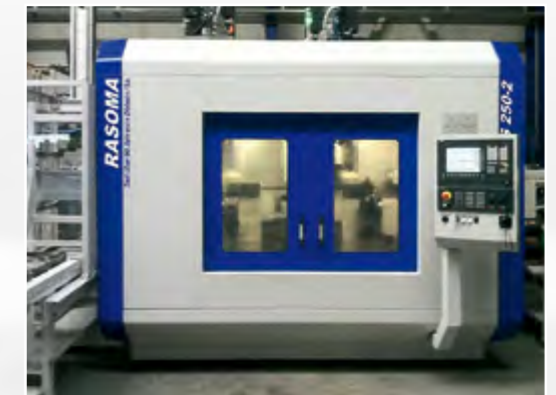
DZS 250-2 with two motor spindles, two compound slides and two 12-fold star turrets for simultaneous processing of OP 10 and OP 20
