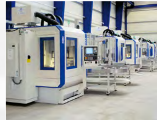
10 DS 250 machines with oval storage, lined up in pairs, for semiautomatic machining of gear wheels for commercial vehicles before and after heat-treating
