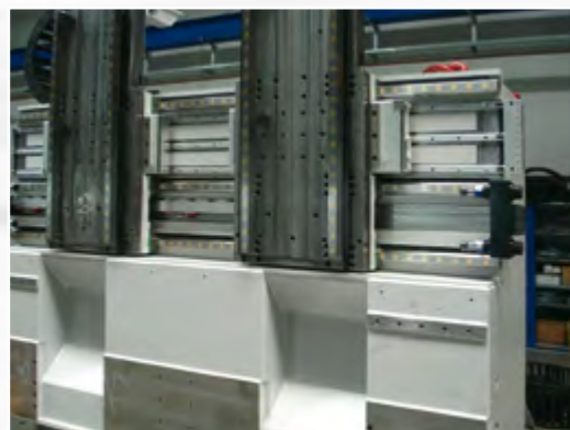
Basic structure of the DZS machines, here with two compound slides on three linear guides with intermediate linear motor
