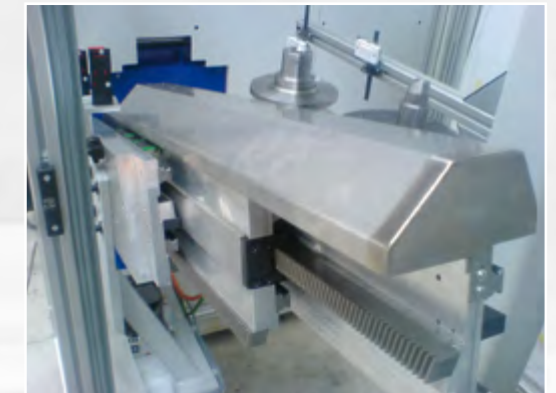
RASOMA telescopic slide for feeding and removal of parts
