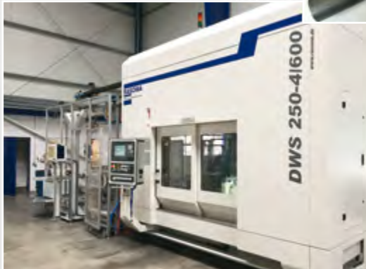
RASOMA vertical- shaft turning center DWS 250-4 with automated loading and unloading for workpieces
