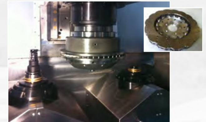
Hobbing of contour at the periphery of a disc-shaped part in DZS 250
