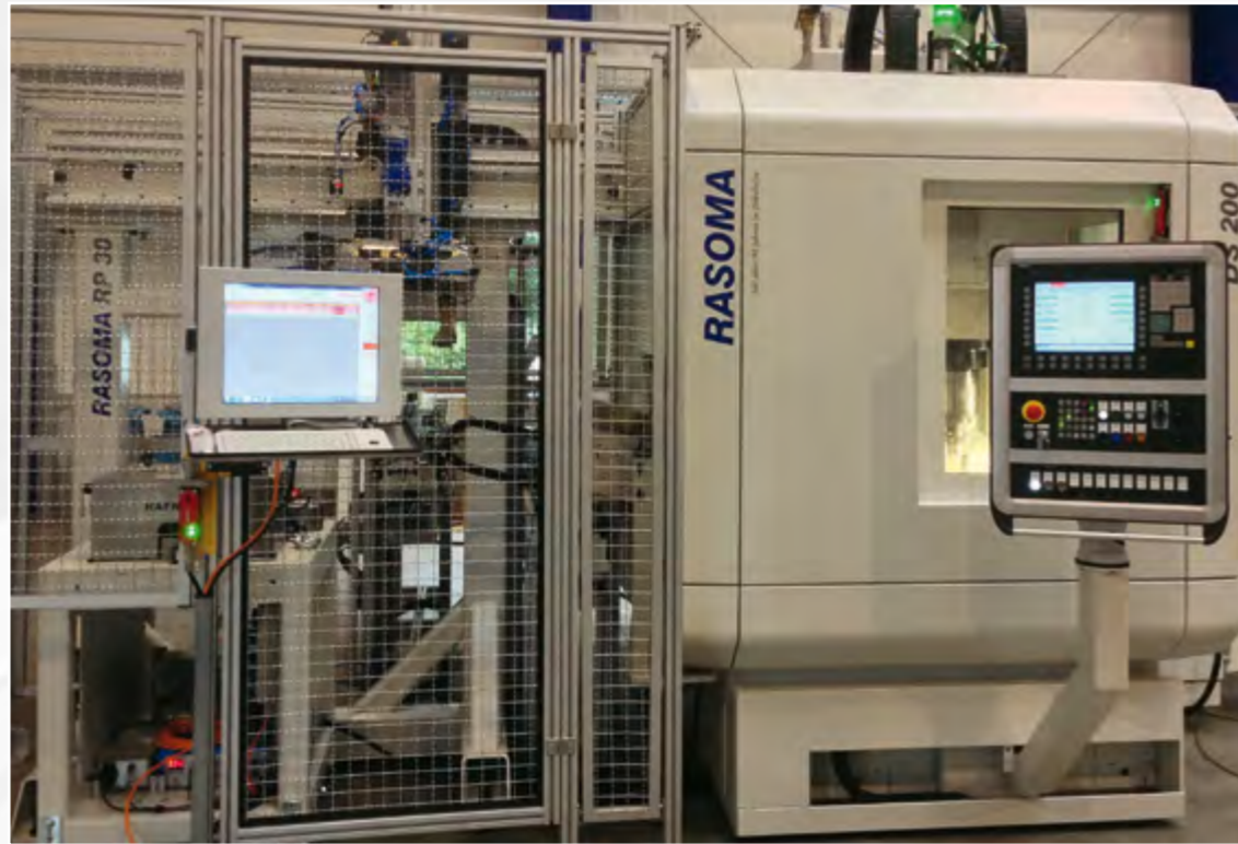
DS 200 with feed and discharge conveyor of work pieces, RASOMA portal RP 30 and external measuring station (coloring as per specification sheet)
