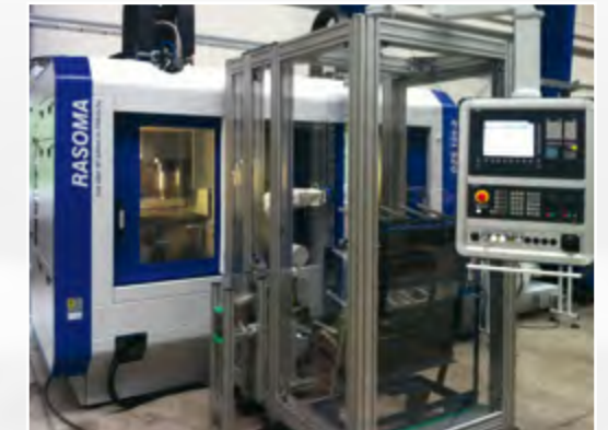
Articulated robot for loading/unloading and feeding of the measuring station, SPC slide and stacking mandrel storage of finish parts
