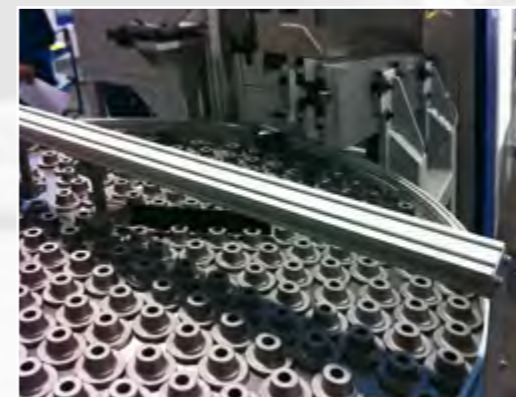
Plate storage for raw parts and telescopic slide with manipulator
