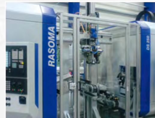
Fully automatic machining of 1st and 2nd clamping operation, turning of the wheel hub to be machined in the gripper
