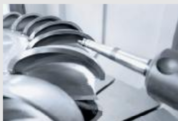
Finishing of a Pelton wheel from a single piece – ø 1,600 mm Complete machining on a DMU 210 FD
