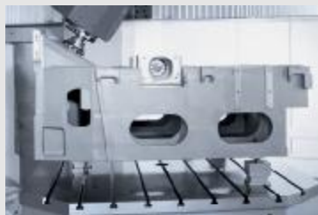
Roughing of a machine column Complete finish machining on a DMC 340 U
