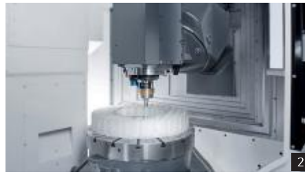
1: Machining a diffuser case from Inconel 718 with an ULTRASONIC 125 FD 2: ULTRASONIC 60 FD duoBLOCK®: Thin-walled, lightweight structures of a Zerodur mirror carrier 3: External / internal cylindrical grinding of a mineral cast pump housing on an ULTRASONIC 125 FD
