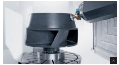
1: Machining a diffuser case from Inconel 718 with an ULTRASONIC 125 FD 2: ULTRASONIC 60 FD duoBLOCK®: Thin-walled, lightweight structures of a Zerodur mirror carrier 3: External / internal cylindrical grinding of a mineral cast pump housing on an ULTRASONIC 125 FD
