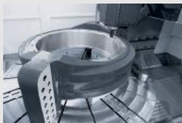
Turning of a bearing housing (wind energy) Complete machining on a DMC 340 FD
