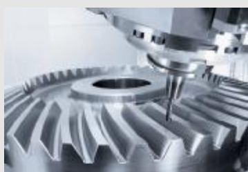
Hard machining of a bevel spur gear (60 HRC) – ø 1,320 mm Complete machining on a DMU 210 FD
