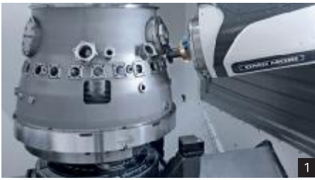
1: Machining a diffuser case from Inconel 718 with an ULTRASONIC 125 FD 2: ULTRASONIC 60 FD duoBLOCK®: Thin-walled, lightweight structures of a Zerodur mirror carrier 3: External / internal cylindrical grinding of a mineral cast pump housing on an ULTRASONIC 125 FD
