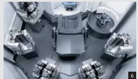
1: DMC U as pallet magazine with a container option 2: Production system with three machining centers, 2-level linear magazine with 52 slots and a central tool magazine with 400 slots (24,000 rpm. HSC pick-up spindle) 3: Production cell for hydraulic components 4: Fully automated production of gear boxes 5: DMC 100 U duoBLOCK® with an RS10 rotary magazine 6: RS5 rotary magazine
