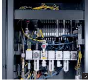
1: Compact 132.1 gal. coolant tank, screen filter and 580.2 psi. internal coolant supply 2: Tool break control during machining operations (mechanical) 3: HSK tool taper cleaning (mechanical) 4: Control cabinet construction according to automotive standards 5: Maintenance-friendly fluid box
