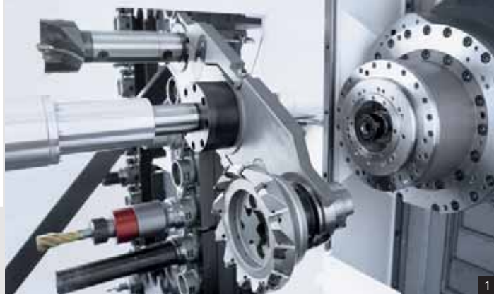
1: Highly dynamic vertical chain magazine for up to 480 tools and fast setup 2: Quick cam-controlled double gripper for unbeatable chip-to-chip times (3.7 sec. with HSK-A63 and 3.9 sec. with HSK-A100)
