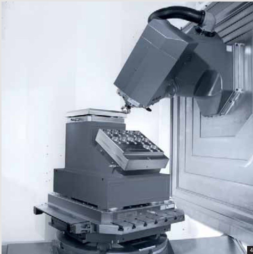
4: Large cubic work area and consistent precision (even in the upper travel range) through 3 X-axis guideways 5: Steep (30°) 1-piece covers in the chip fall area 6: Quick chip disposal to the rear
