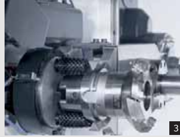
1: Compact 132.1 gal. coolant tank, screen filter and 580.2 psi. internal coolant supply 2: Tool break control during machining operations (mechanical) 3: HSK tool taper cleaning (mechanical) 4: Control cabinet construction according to automotive standards 5: Maintenance-friendly fluid box
