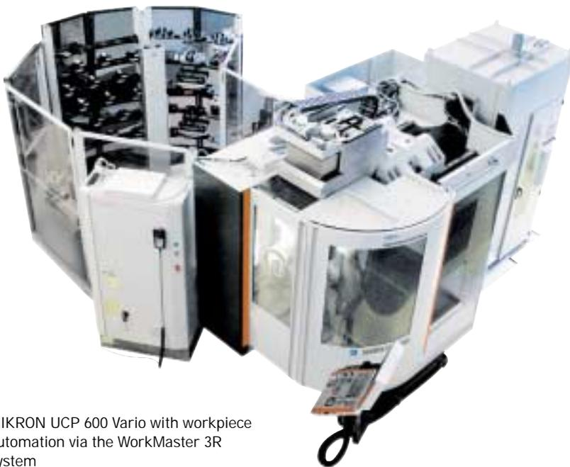
MIKRON UCP 600 Vario with workpiece automation via the WorkMaster 3R system
