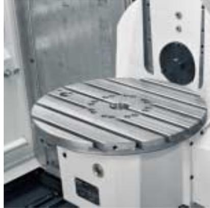
Rotary tilting table with parallel grooves
