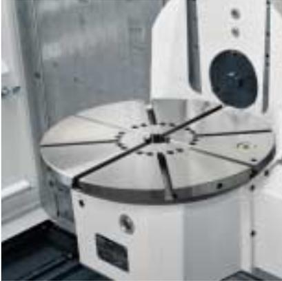
Rotary tilting table with radial grooves
