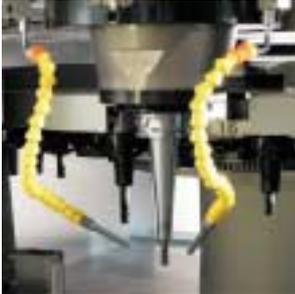
Minimum quantity cooling lubrication
