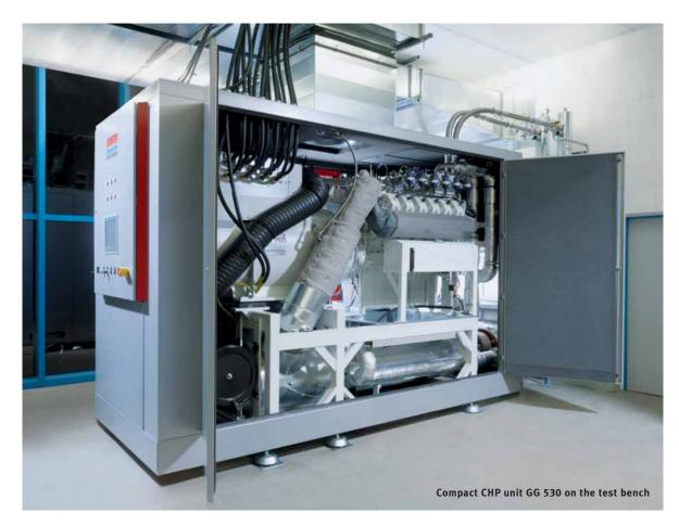
Core piece of the CHP unit is a gas engine which powers an alternator. The cooling water and exhaust heat are extracted with a system of heat exchangers and transferred to heating water. Engine, alternator and base frame are mounted with multiple vibration dampeners, the casing with integrated switchgear is fully sound-insulated.
