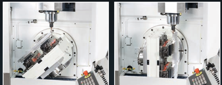
Clamping table U4-1520 Clamping surface on both sides
