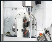
Clamping table U4-620 Clamping surface on both sides
