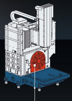
All versions with modern linear guides on rigid cast construction
