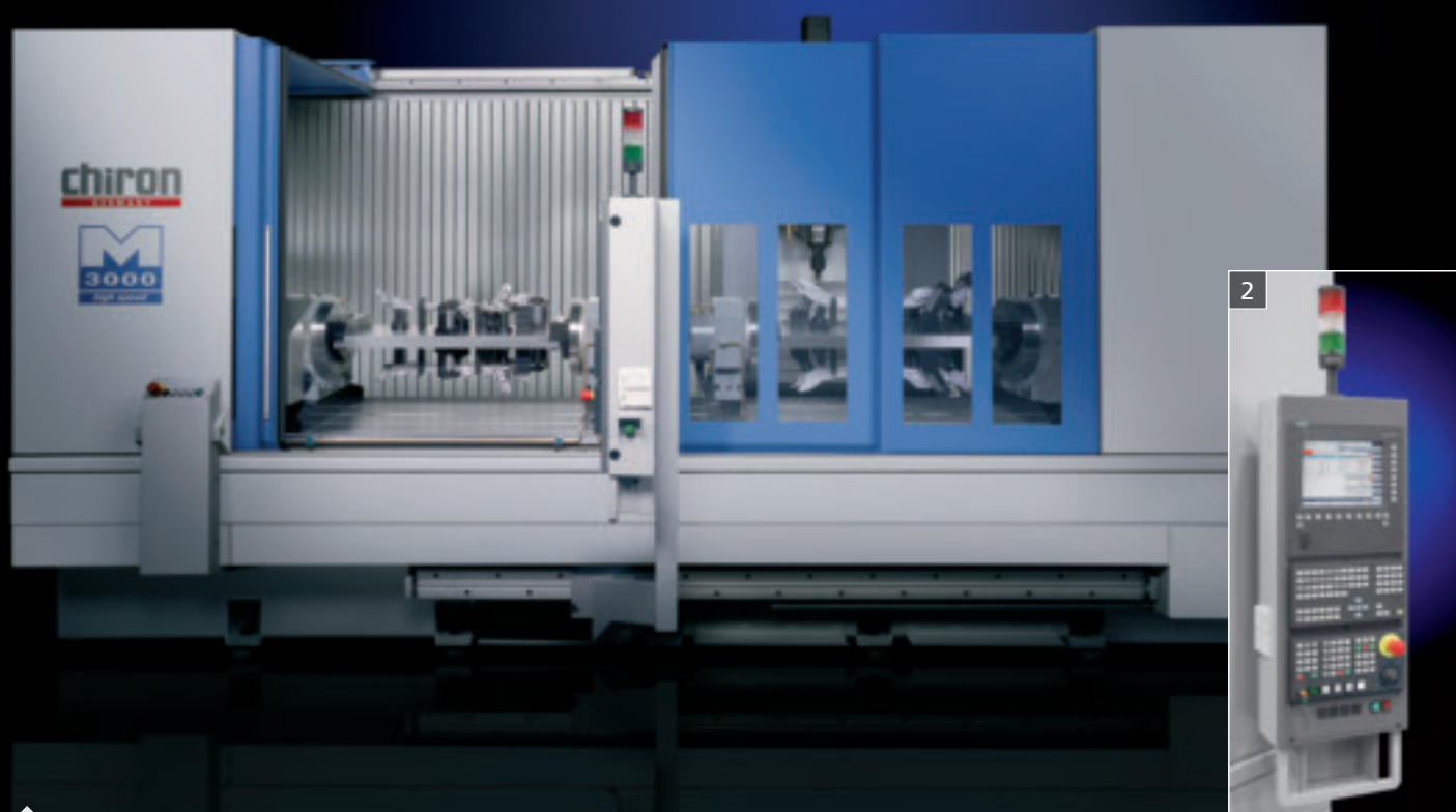
MILL 3000: Pendulum mode with inserted, chip-proof central splash guard
