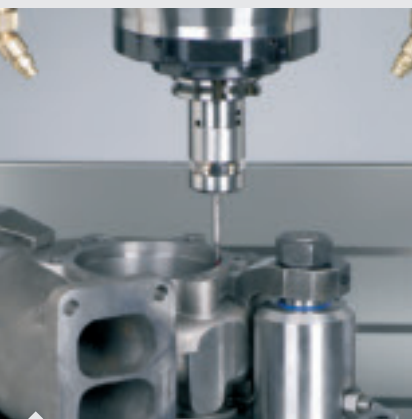
Machine integrated workpiece measurement by using a 3D probing system
