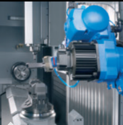
Space saving integration of an articulated arm robot for removing finished parts
