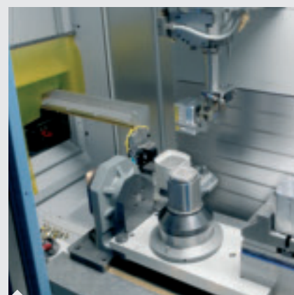
Spindle gripper for machine-integrated workpiece handling
