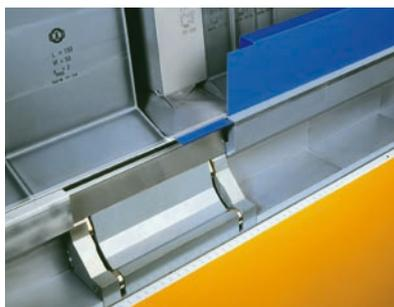
UpDown-tool inactive position (collapsed)
