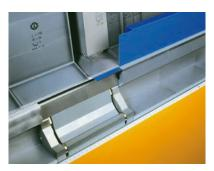
UpDown-tool inactive position (collapsed)
