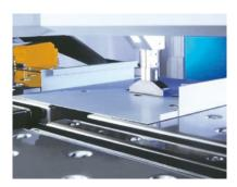
The main manipulator positions and rotates the blank with an accuracy of 0.001 degree.
