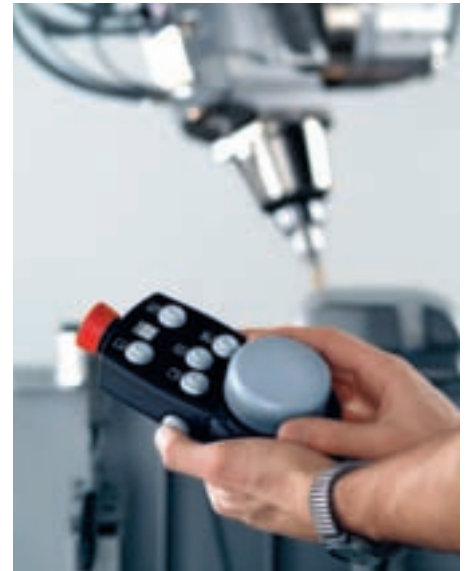
Rapid run-in and teach-in using the 6D mouse.
