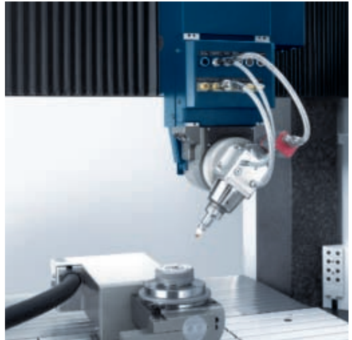
The focusing optics can be quickly interchanged on the swivel axis.
