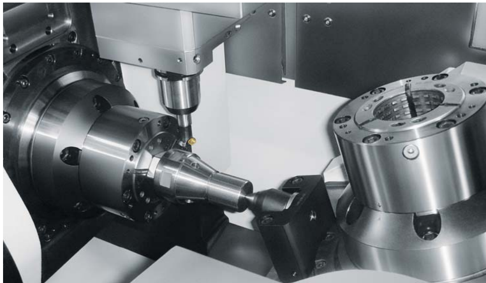
Work area MC 734/MT with powered tailstock center and counter- spindle with chuck or jaw chuck.
