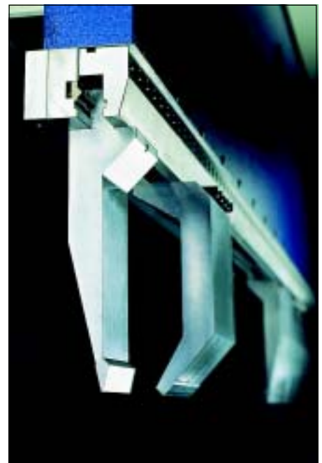
Comfortable: self-centering punch holder
